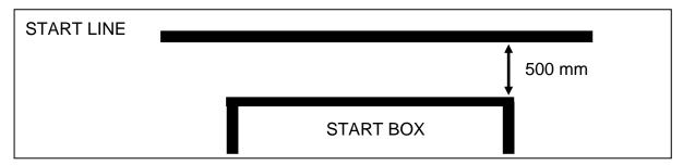
The start line and start box are marked at the start. The start beam is located at the Start Line. The start box is positioned 500 millimeters behind the start line.
